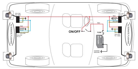
The front and rear heads are configured to flash independently of each other. In order to have the front and rear heads flash in sychronization, the blue wires from all units must be connected. The yellow wire can then be used to determine either alternate or simultaneous flash between each unit in the system by connecting to either power or ground.
