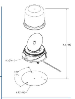
45° angled reflector driven by a quiet brushless magnetic drive—system provides an exceptional warning beam without compromising reliability
