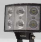
EW2530 SIX 10-WATT LEDs 12-24V | Flood | 3,750 Lumens Deutsch connector | 120° beam pattern CE, R10, CISPR25, IP67, IP69K, RoHS
