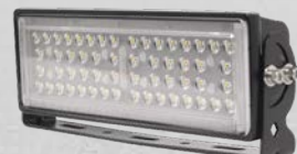
EW4030 FIFTY-SIX 1.5-WATT LEDs 12-24V | Flood | 4,950 Lumens Deutsch connector | 170° articulated mount CE, R10, IP67, RoHS
