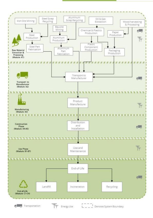
**Figure 1.** Flow diagram representing the major unit operations in the life cycle of the Skyfold Zenith® products.
