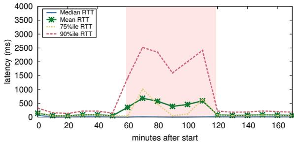
(c) Experiment H: 90% packet loss (1800s TTL)
