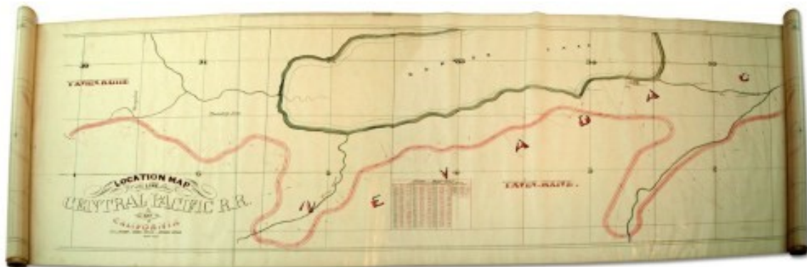
Judah's original concept for twin ascending turns in Coldstream Cañon and Strong's Cañon, just west of Truckee. These allowed the line to climb 828 vertical feet, on its way to the 7,046 ft high Donner Summit. Part of 66-foot map. (California State Archives)
