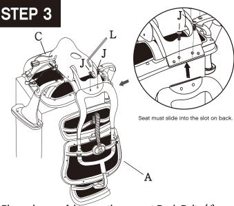
Please be careful to use the correct Back Bolts (J). Assemble the Backrest (A) to the Seat Cushion (C) using 2 Back Bolts (J).
