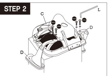
The <u>Type B Arm Bolt is shorter</u> and will be inserted into the hole CLOSER to the mechanism. The <u>Type A Arm Bolt is longer</u> and will be inserted into the hole FARTHER away from the mechanism.
