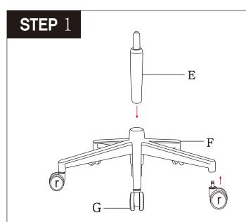
Press the Casters (G) into the holes at the end of each leg of the Base (F).
