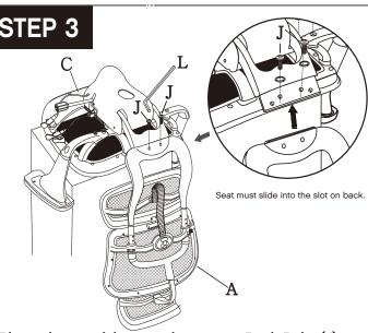
Please be careful to use the correct Back Bolts (J). Assemble the Backrest (A) to the Seat Cushion (C) using 2 Back Bolts (J).
