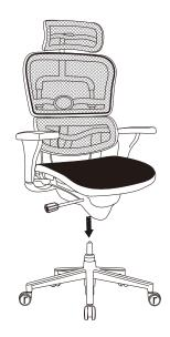
Now turn the assembled seat upright and locate the center hole of the Mechanism over the Seat Post. Push down firmly until the connection is secure.
