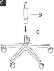
Please insert the Seat Post (B) into the center hole of the Base (C).
