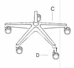
Please press the Casters (D) into the holes at the end of each leg of the Base (C).
