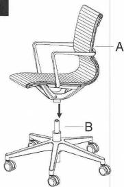
Now turn the assembled seat upright and locate the center hole of the mechanism over the Seat Post (B). Push down firmly until the connection is secure.
