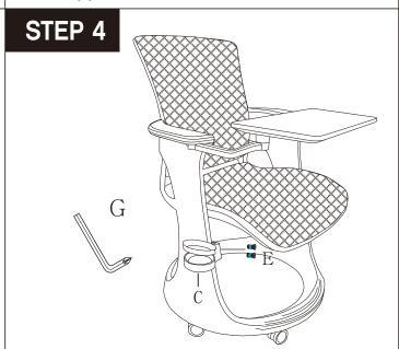
Please be careful to use the correct Cup Holder Bolts (G). Assemble the Cup Holder (E) to the storage shelf using the Cup Holder Bolts (G).
