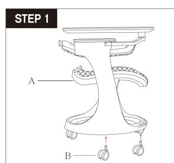
Press the Casters (D) into the holes at the bottom of the Base and Seat Cushion (A).
