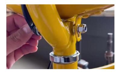
4. Screw the nuts back on and tighten them securely using a wrench. Make sure the mudguard is firmly in place and that no parts are loose.
