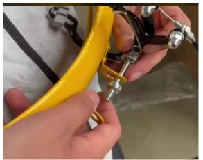
2. Assemble the mudguard between the front fork and the frame, ensuring that the holes on the mudguard align with the hole on the front fork.
