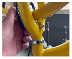
3. Insert the bolt through the hole in the mudguard and then through the hole in the front fork. Reattach the washers you removed in step 1.
