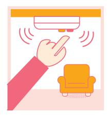
Install the smoke alarms in the middle of the ceiling in each room (excluding kitchen and bathroom). One alarm for each 60 sqm of floor space is enough. If your home has more than one storey, install a smoke alarm in each storey.
