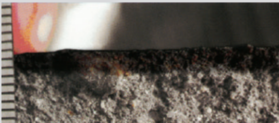
Siplast Primer® Speed SBS: 2–3 mm
