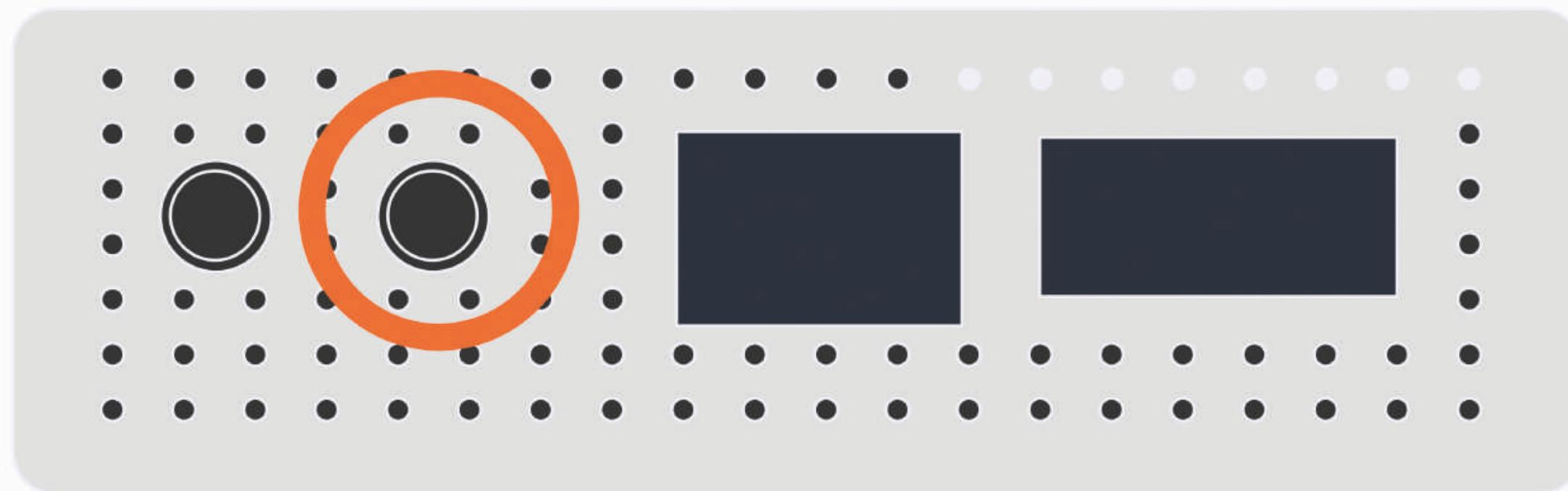
Make sure the signal cable from the fusebox is properly connected to the Watty box. There should be a distinct “click” when it connects.
