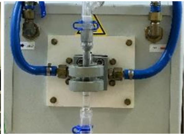
General view of the laboratory pilot plant (D) and close-up of the reactor with the injection coil and cooling system (G).
