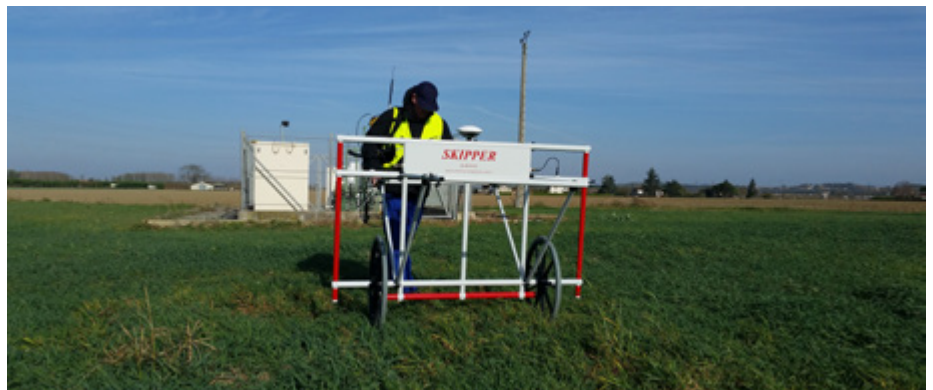
Magnetic tomography inspection of pipelines in conjunction with specialist contractor, Skipper.
