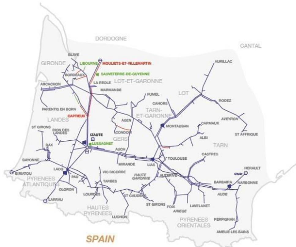
TIGF's network has 6 compression stations with a total power output of 70 MW. 2014 annual gas consumption in the area served by the TIGF network amounts to 31 TWh, compared to a total of 450 TWh of annual gas consumption in France.
