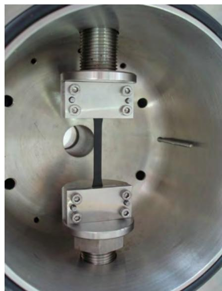
Hydrogen pressure chamber with tensile specimen.
