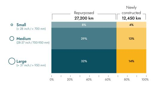
Figure 5 shows that, based on an analysis of the existing gas network, almost 90% of the European Hydrogen Backbone can be expected to consist of medium (28-37 inch, 700-950 mm diameter) and large (> 37 inch, > 950 mm diameter) pipelines. For simplicity, it is assumed that the share of pipeline diameters for newly built hydrogen stretches remains comparable to the current shares in the natural gas network.
