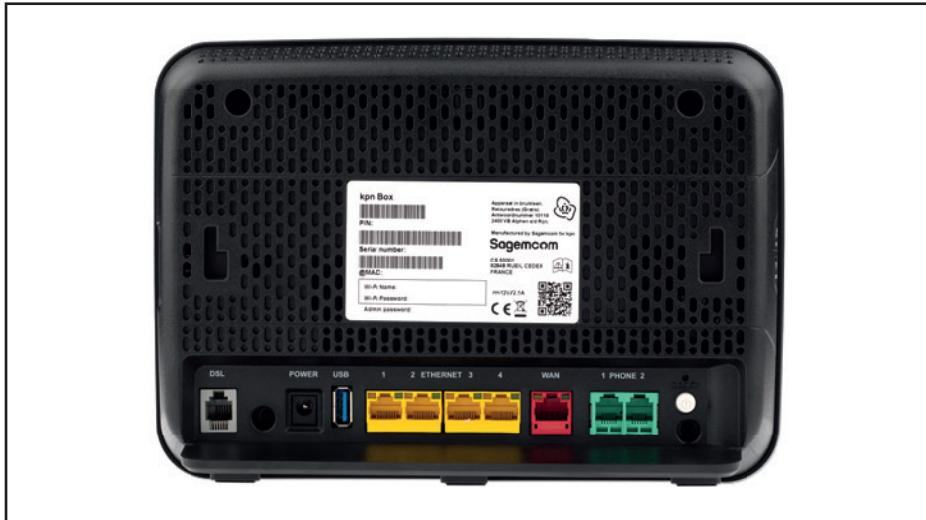
**On the back of the modem, you will find the connection points at the bottom. From left to right**
