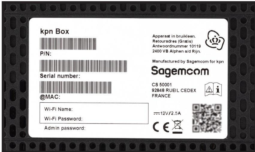
There's also a QR code on the back of the modem that contains all the modem's Wi-Fi information and login details. Your smartphone can scan this QR code with its camera and decipher the codes. This is useful because copying and pasting this information prevents errors.
