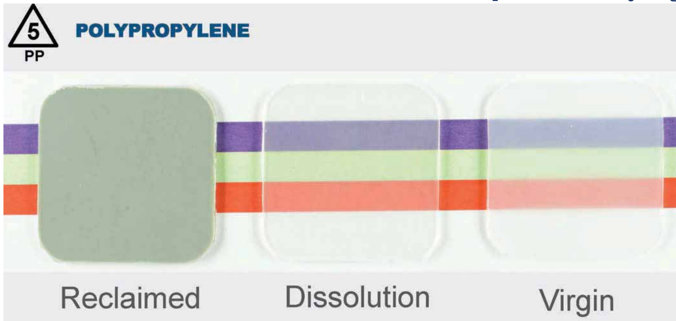
Figure 2: Comparison dissolution recycling of PP and PE with virgin plastic
